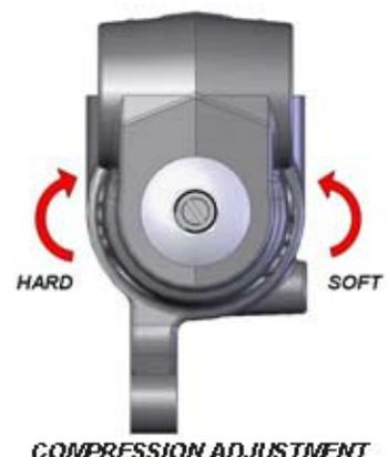
At the base of the conventional leg is another adjustment screw that controls the amount of compression damping. Turning this screw clockwise increases damping and turning it counter-clockwise will decrease it. This is illustrated by the “HARD” and “SOFT” in the figure at the right.
