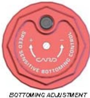
The Smart Leg cap is labeled “Speed Sensitive Bottoming Control”, and this adjuster provides a range of control over how progressive the fork feels. Turning the screw clockwise increases the fork’s resistance to bottoming, while turning the screw counter-clockwise decreases it. On the track, this effect will be felt on sections where the fork is forced to move very quickly such as on harsh landings or when traversing sharp edged bumps.
