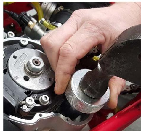
**NOTE:** It may be necessary to tap the outer bearing race in (hammer & blunt punch) or out (with slide hammer) to insure proper free operation of the shaft while the screw is tight.
