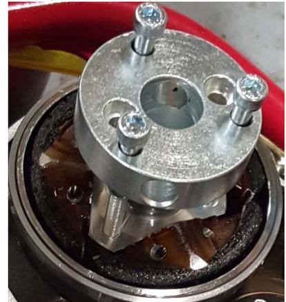
**NOTE:** It may be helpful to use a screwdriver or similar device in the side hole of the puller to stop rotation
