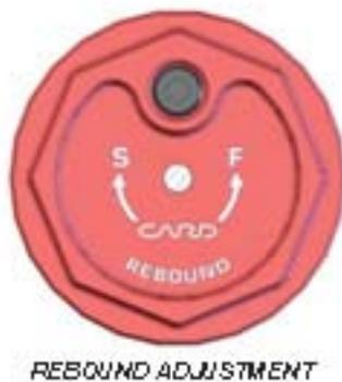
The speed at which the fork rebounds can be adjusted at the top of the conventional leg. Turning the adjustment screw clockwise slows the rate at which the fork extends after being compressed, and likewise, turning the screw counter-clockwise returns the leg to its extended position faster. As shown in the figure, 'S' (slower) and 'F' (faster) are etched into the cap as an adjustment guide.
